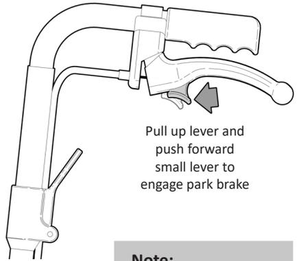
Pull up lever and push forward small lever to engage park brake
