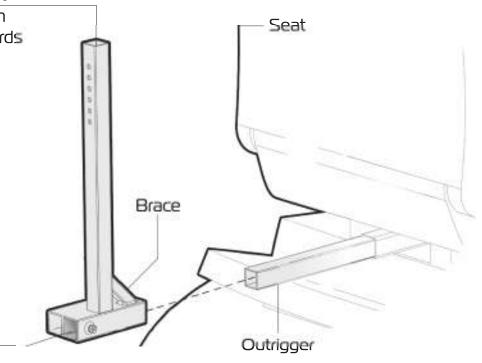
Slide the tube — underneath the vertical tube onto the outrigger.
